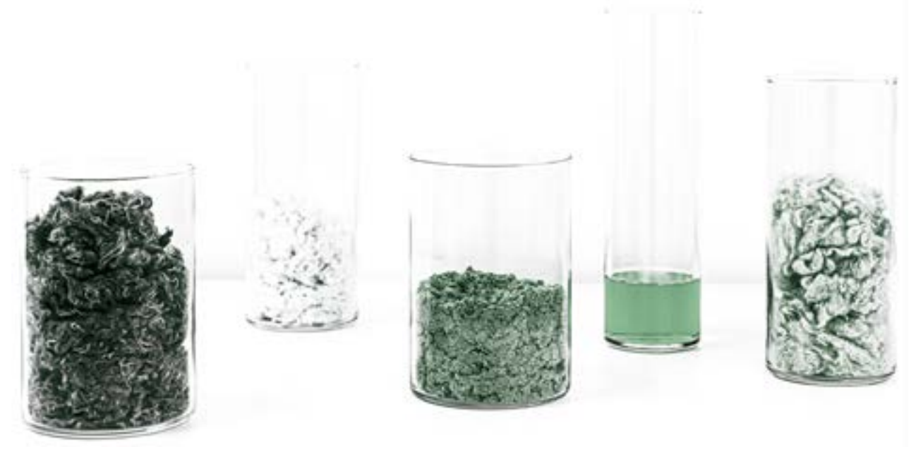
Image of the process in glass jars (when using textile waste as the raw material). From left to right: shredded textile waste (someone’s old jeans); the remaining cellulose after non-cellulosic materials like polyester, dyes and textile finishing chemicals have been removed; cellulose carbamate powder (the result of the magical bit of the process, carbamation, where the cellulose reacts with urea); dissolved carbamate powder which is wet-spun to create the product in the final jar; cellulose carbamate fiber, known as Infinna™, which has the natural, soft look and feel of cotton and unique characteristics, including superior dye uptake and naturally occurring antimicrobial properties.
